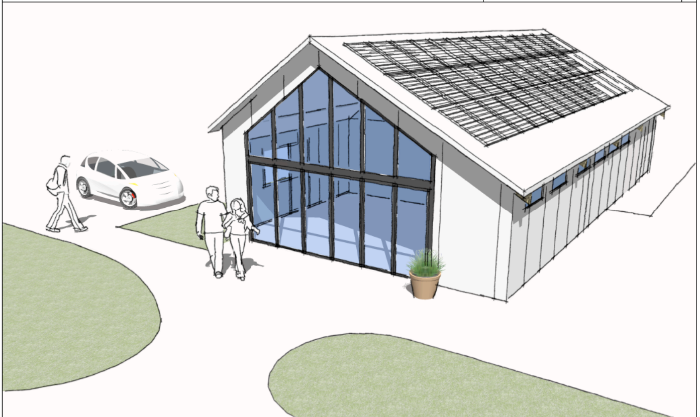
View of proposed building from West, showing extensive gable end glazing and solar panels
